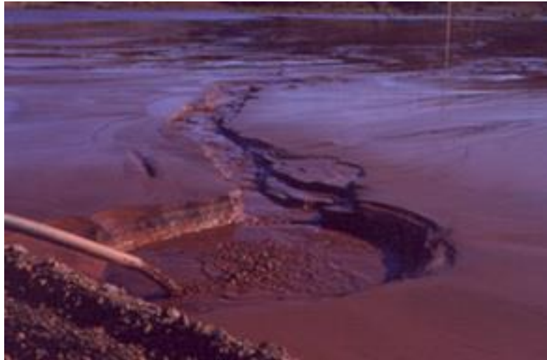
Figure 2: Conventional Tailings Slurry Disposal (Australian Government, 2016)
