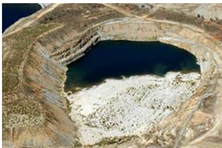
Figure 4: Co-Disposed Waste Rock and Thickened Tailings in a Completed Open Pit (Australian Government, 2016)
