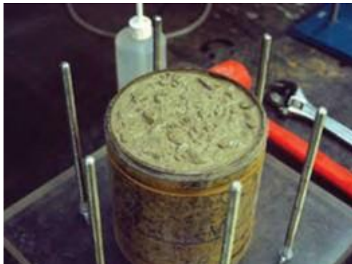
Figure 5: Integrated Coarse and Fine Wastes in the Laboratory (Australian Government, 2016)
